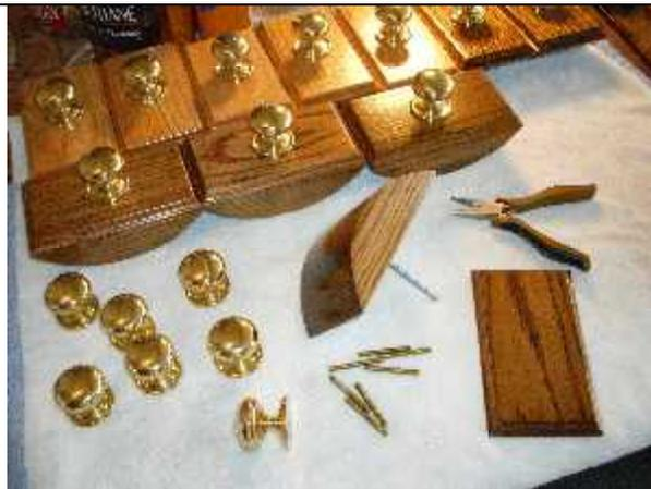
**29.** Temporary zinc studs are replaced with brass studs and topped off with a Liberty solid brass knob.
