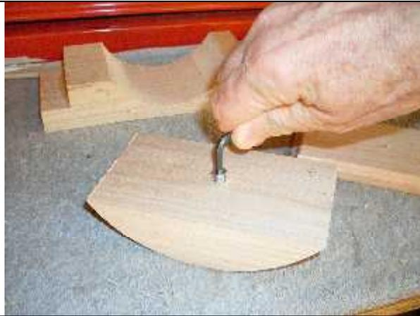
17. Insert nuts are screwed into place using an allen wrench.
