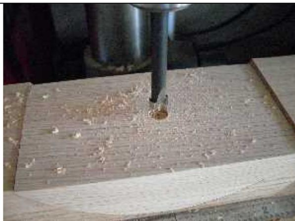
**15.** The top 1/16<sup>th</sup> of the hole is widened to counter sink the insert nut.
