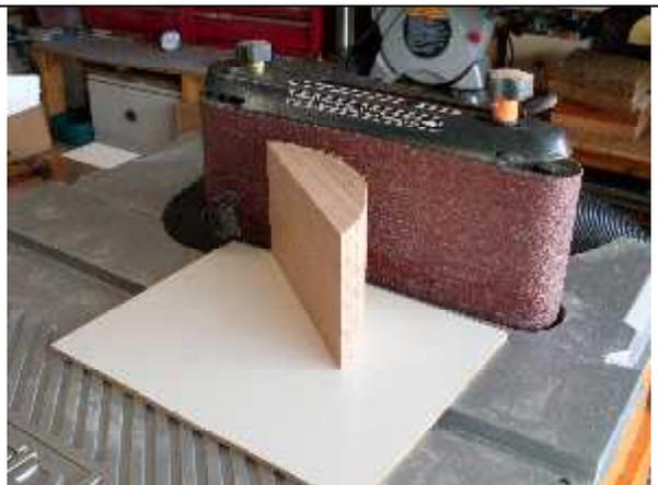
7. An oscillating belt sander is used to smooth out the bottoms. This process takes 10 to 15 minutes for each rocker.
