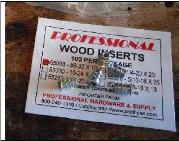
16. Insert nuts are used to anchor the brass knob post.
