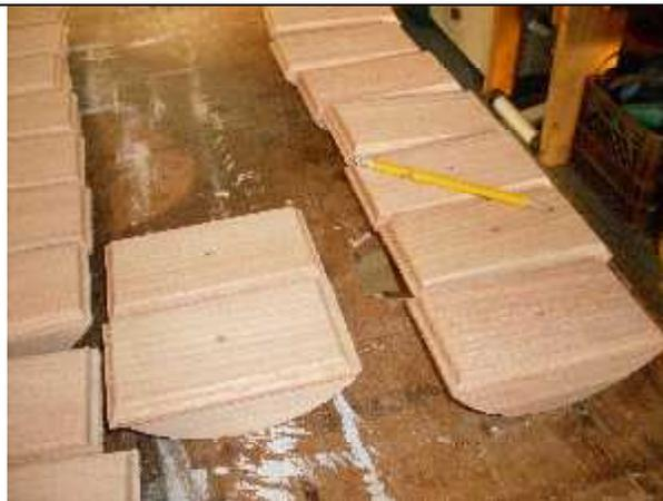
18. Paired tops and bottoms are numbered to keep them together through the sanding process.
