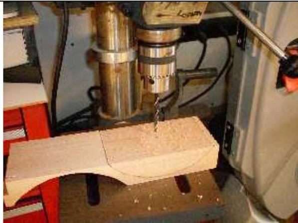
**14.** Holes for insert nuts are drilled. Scrap cutouts are used to stabilize and center the rocker bottom.
