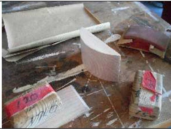
19. Tops and bottoms are hand sanded at 120 grit, inspected for scratches, then sanded again at 150 grit, and re-inspected for scratches, and given a final sanding at 180 grit.
