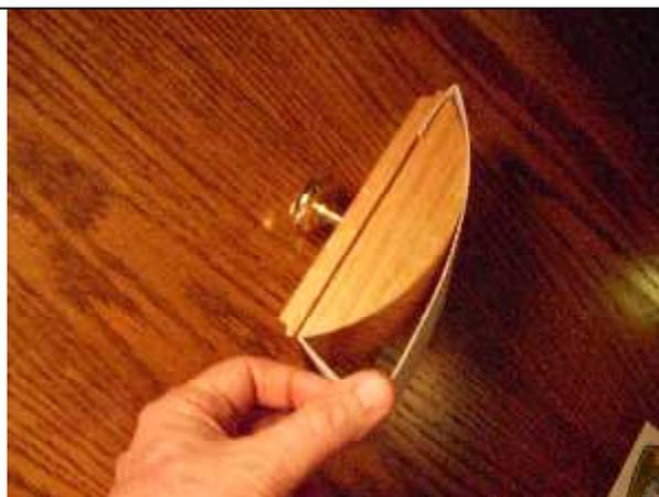
**30.** The brass knob is loosened, blotter paper is fitted and the knob is retightened and you are ready to go.
