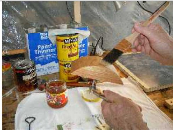
25. All tops and bottoms, both stained and natural, are brushed with a sealer coat of 50% polyurethane varnish and 50% paint thinner.
