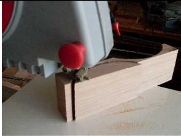
5. Rockers are rough cut on a band saw.
