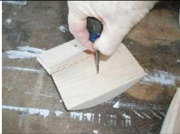
**13.** Using the top as a template the hole for the insert nut is marked.
