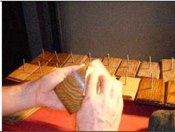
**27.** After the sealer coat all pieces are lightly sanded with 600 grit paper. Then each top and bottom receives 3 top coats of polyurethane varnish. The thick top coat will protect them from inks and naturally occurring body oils from the hands. They are easily cleaned with a slightly dampened cloth or a liquid polish if you prefer.
