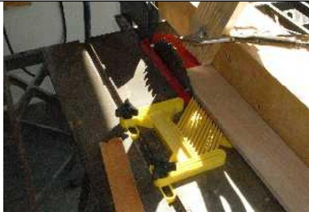
**9.** Tops are  $\frac{1}{2}$  oak stock and cut to width, matching the width of the rockers.
