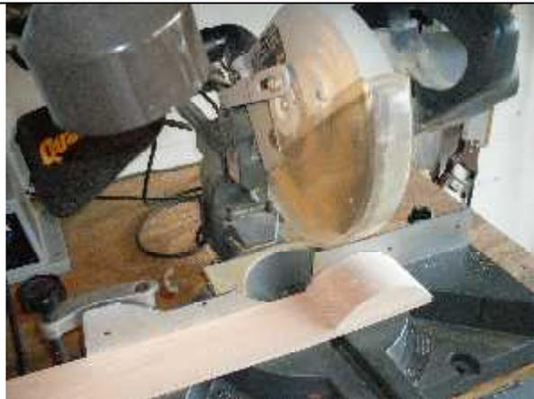
**10.** Tops are cut to match the length of the rockers. Each set of top and rocker bottom are individually matched.
