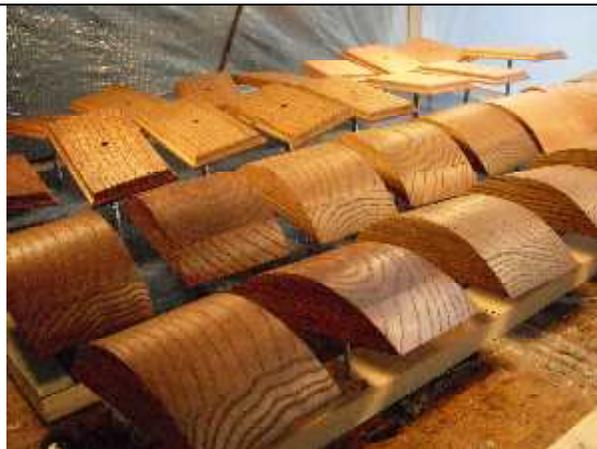
26. Drying time is at least 8 hours between sealer coat and each successive top coat. Rocker blotters dry in a dust free tent.
