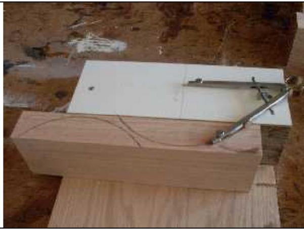
4. The length of the arc will cover a personal check in one motion. This simple jig helps provides a nearly consistent pattern for the next step.
